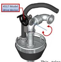
This telescopic drop tube is manually operated by a handwheel device (C-4517) and it can be realized with 2 or 3 sections. In order to extend it, it is necessary to unlock the stop lever, then act on the handwheel that, through 2 ropes, extends the telescopic tube. At the end of loading, operations and after locking the device with the stop lever, it is sufficient to act on the handwheel on the opposite direction in order to close the telescopic tube.
