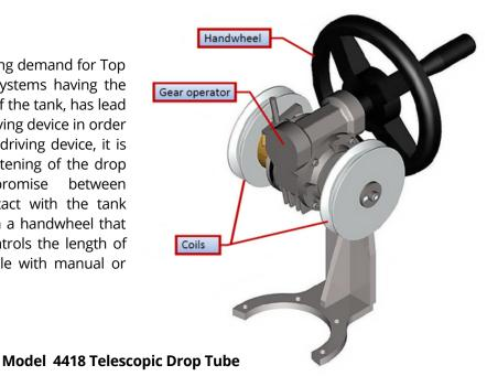
The telescopic drop tube is a special vertical tube installed on Top Loading Arms with vapour recovery system, with adjustable length device. This device makes it possible to extend/shorten the drop tube. This is a good compromise between easy manoeuvrability and the necessity to touch the bottom of the tank, in order to guarantee a continuous conductive patch.
