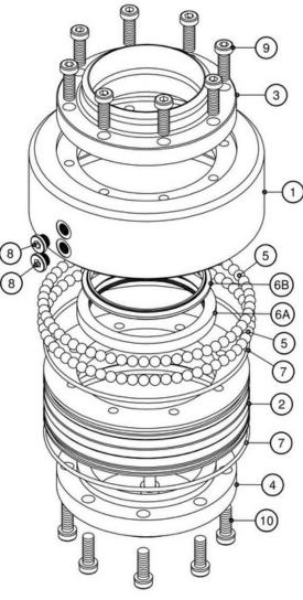
The Model 3996-WN with butt weld flanges is a 4 piece design with hardened and ground raceways with a reduced height which makes it suitable for bottom unloading. It has a primary seal "C" profile. The design allows for a quick Swivel Joint replacement and easy swivelling/seal replacement.
